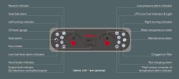
Reliable dashboard shows the truck's working condition, faults and other important information for convenient operator control
