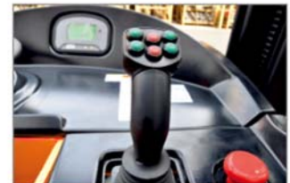
Control handle with integrated thumb stick, allows smooth operation of (1) Travel, (2) Lift/low, (3) controls Tilt and Fork Reach.
